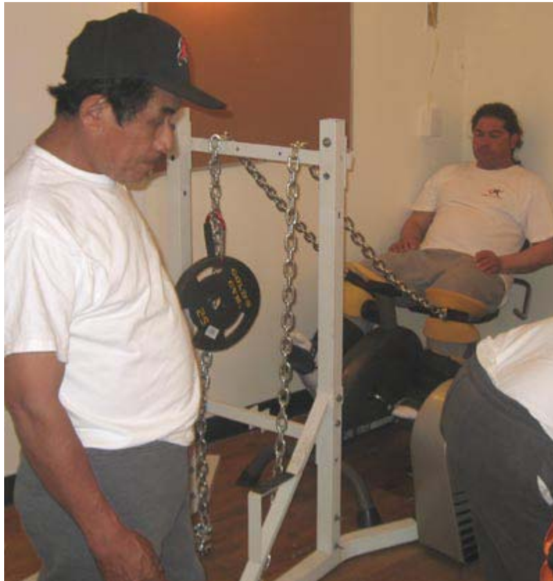
We tested with chains and learned that they cause too much friction and noise. Our advice? Stick with nylon ropes.
